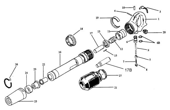
Note: K800 and K1100 purchased after May 2003 are equipped with the new style retained piston and cylinder
